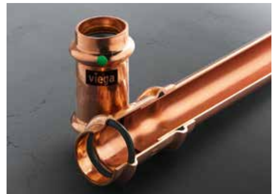
Clear marking: Press connectors marked in green have been factory-fitted with the EPDM sealing element.
