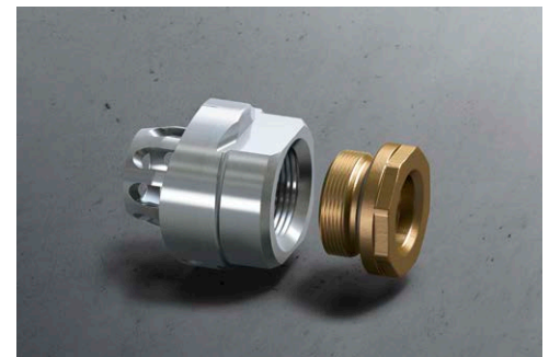
The press-in branch connector is suitable for steel pipes in accordance with DIN EN 10255, DIN EN 10220/10216-1 or DIN EN 10220/10217-1 and available for steel pipe sizes 1½, 2, 2½, 3, 4, 5, and 6 inches. It is provided with an Rp ¾-inch internal thread. A reducer to an Rp ½-inch internal thread is additionally available.
