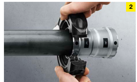
For pressing Megapress connectors from 1\frac{1}{4} inch upwards, only press rings with hinged adapter jaws are used. For smaller sizes between \frac{3}{8} and 1 inch, both press jaws and press rings with hinged adapter jaws are available.
