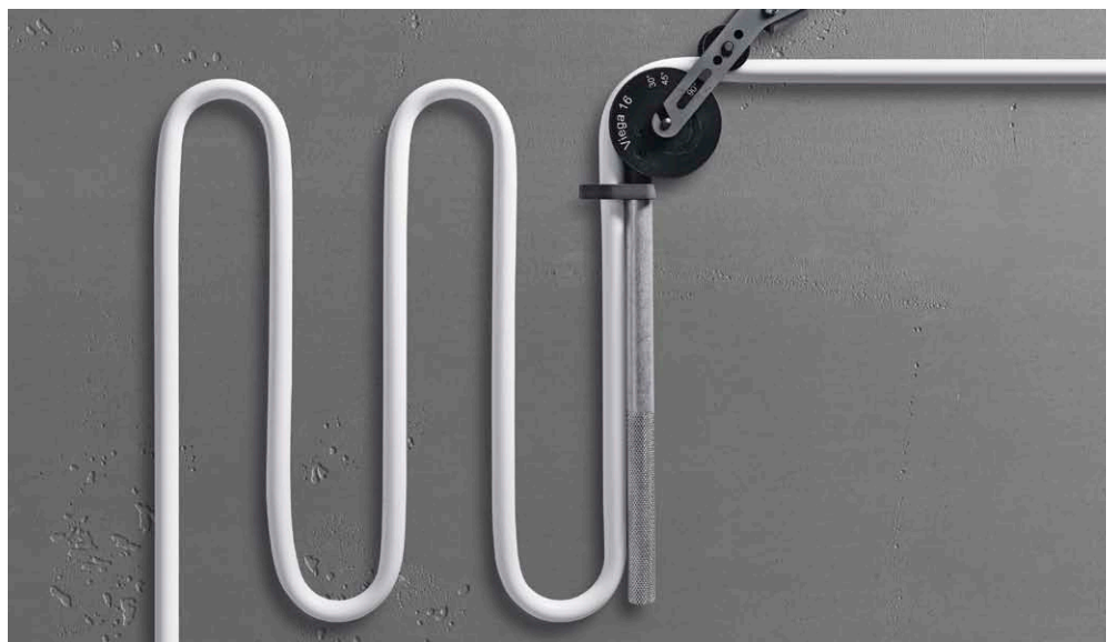
The bending tool can be used to easily create perfect radii.
